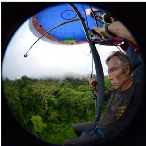
Fig. 3: The “Cinébulle” is a hot air balloon allowing to collect samples and conduct observations in the forest canopy. It is the only technique allowing to reach the canopy surface.
