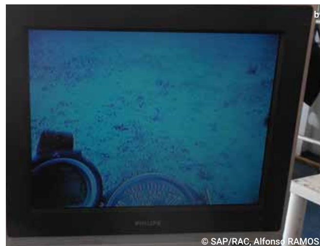
Figure 3.5. ROV 'Prometeo': a) On the surface of the water before sinking; b) display on deck showing the seafloor (73 m depth).
