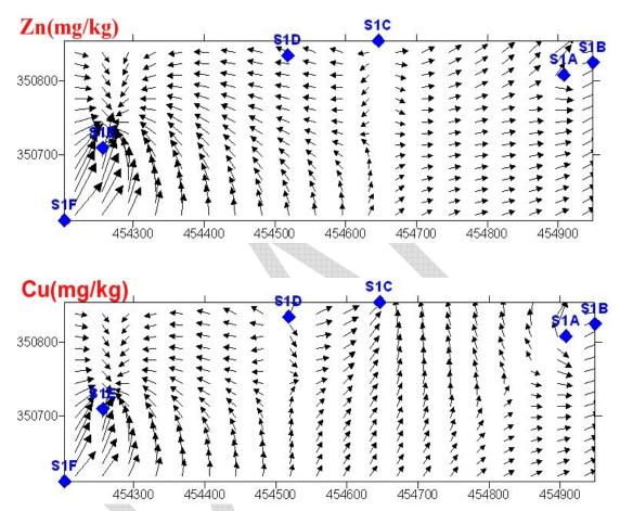
Figure 3: Vector maps of Zn & Cu in sediments of Darbandikhan Lake showing input (winter survey)
