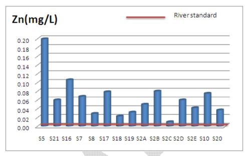
Figure 20: Concentration of zinc in water samples of Little Zab River Watershed (Dukan Basin)
