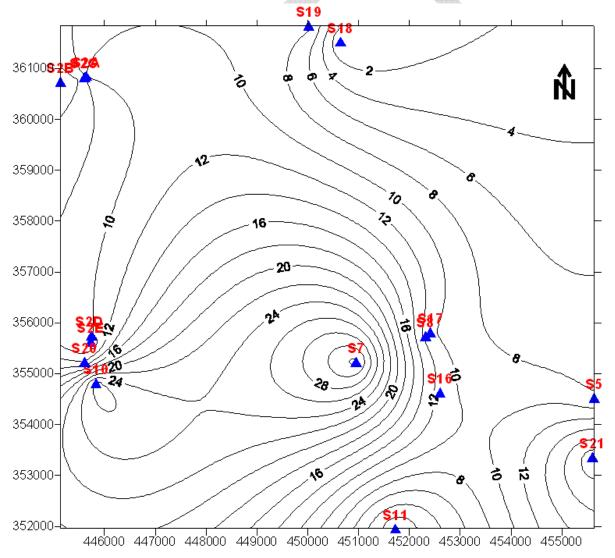
Figure 5: Concentration distribution map of magnesium in water samples of Little Zab River Watershed (Dukan
