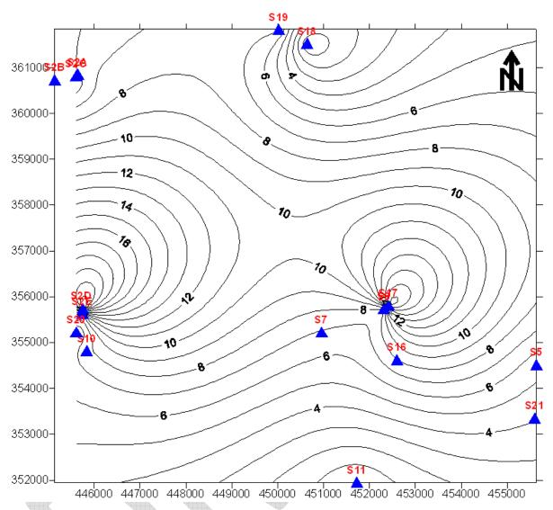
Figure 9: Concentration distribution map of sodium in water samples of Little Zab River Watershed (Dukan Basin)
