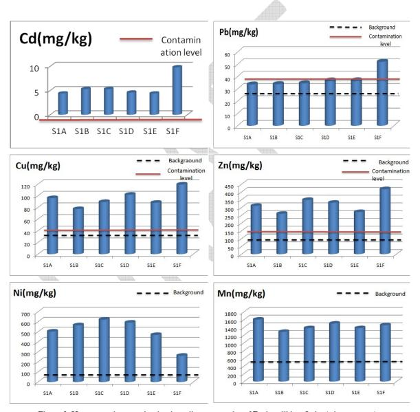
Figure 2: Heavy metal contamination in sediment samples of Darbandikhan Lake (winter survey)
