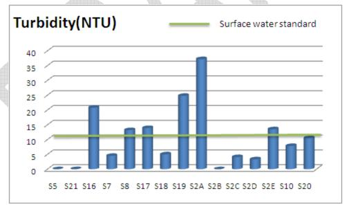
Figure 8: Turbidity in water samples of Little Zab River Watershed (Dukan Basin)
