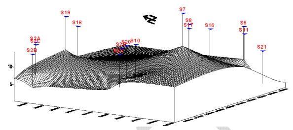
Figure 7: 3D concentration distribution map of cadmium in sediment samples of Little Zab River Watershed (Dukan Basin)
