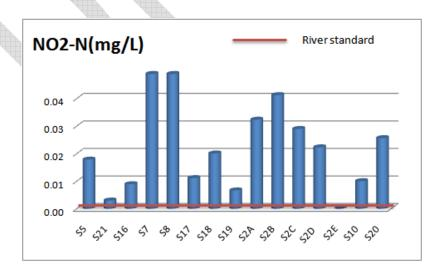
Figure 14: Concentration of nitrite-nitrogen in water samples of Little Zab River Watershed (Dukan Basin)
