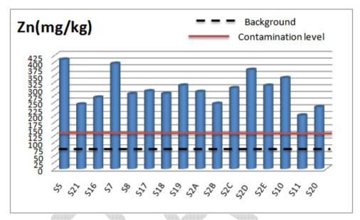
Figure 4: Concentration of zinc in sediment samples of Little Zab River Watershed (Dukan Basin)
